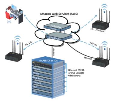
Management ports through Active Standby or Dual Network Access modes. Virtual Router Redundancy Protocol (VRRPv3) enables a group of devices to form a single virtual device to provide network redundancy. The dual AC power supply ensures that console management is available even if the primary AC power source fails. And, protection against electrostatic discharges and power surges is provided with robust 15Kv ESD protection circuitry on each console port.
